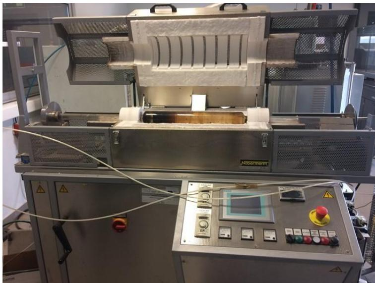
*Figure 3. Laboratorial rotary reactor for torrefaction*
